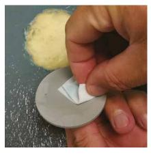
**Important.** Use the supplied adhesive Epoxy 2K. Read the instructions supplied with the glue! From each tube squeeze the same amount. Mix well about 1 minute. The transducer is applied onto the mixed adhesive and pushed hard on the location of the bonding. The glue achieves hold within a few minutes. Stabilize with a cross of adhesive tape (recommended). Adhesive reaches its strength after 1h. **Leave it to dry for min. 1h at 20 deg. C.**!
