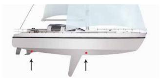
Transducer is installed on the inner side of the hull. It has to be installed on the location, where there is no additional reinforcement of the hull and no shaft bearer 20-30 cm around. If you have a "sandwich" hull, you will need to remove a small section of inner core allowing the transducer to make contact with the outer skin of the hull.
