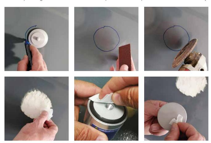
**Important.** Use the supplied Epoxy 2K adhesive. Read the instructions on the adhesive! From each tube squeeze the **same** amount. Mix well for about 1 minute. The transducer/adapter is applied onto the mixed adhesive and pushed hard on the location of the bonding. The glue achieves hold within a few minutes.
