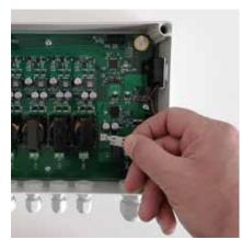
Run the transducer cable through the cable thread and connect it to the terminal blocks. Polarity is not important. Connect 12/24V supply voltage and push the DC connector back in. **Polarity (+/-) is important!** Use 4mm/2 (AWG12). For lengths greater than 10m (30Ft) use a larger cross section.
