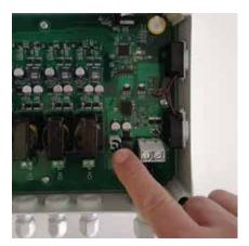
Connect LCD cable strip and close the cover. Press ■ button to turn the device ON and continue with the device settings.
