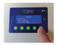
Use ■ button to turn the device ON. Press and hold for 3 seconds to power the device OFF.
